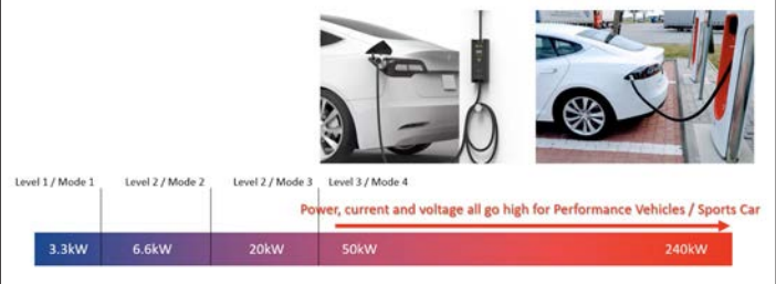
Figure 2. Power requirements for the various levels of automobile battery charging
